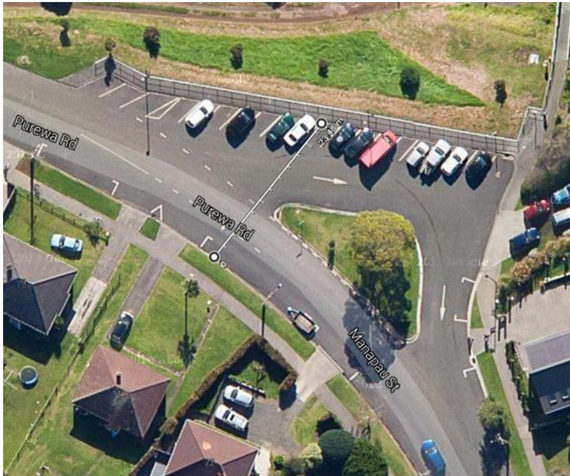
Fig 2. Meadowbank Train Station turning circle is over 23 m wide at its apex 9 .
